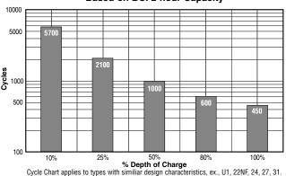
The solar battery excels in cycling applications. \*Dependent upon proper charging and ambient temperatures.
