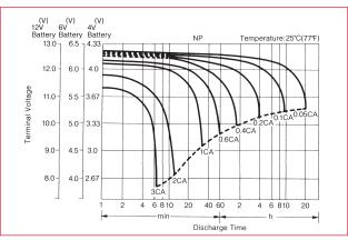
Figure 3. Discharge Characteristic Curves: Genesis NP Batteries
