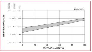
Figure 6. Open Circuit Voltage vs. State of Charge
