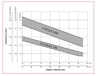
Figure 12. Relationship Between Charging Voltage and Temperature
