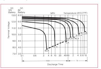
Figure 4. Discharge Characteristic Curves: Genesis NPH Batteries
