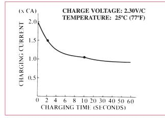
Figure 11. Constant-Voltage Charge Characteristics with no Current Limit
