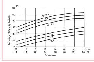
Figure 8. Temperature Effects in Relation to Battery Capacity
