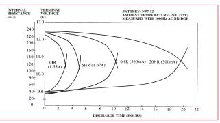
Figure 7. Internal Resistance of NP Battery
