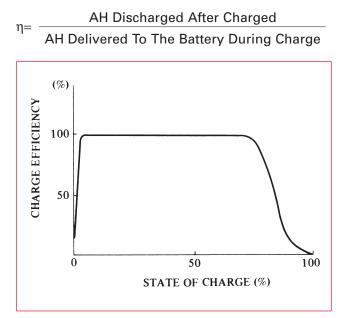
Figure 13. Charging Efficiency vs. State of Charge
