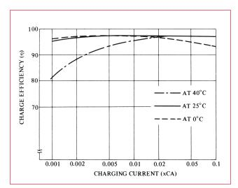
Figure 14. Charging Efficiency
