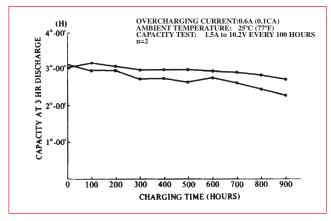
Figure 9. Overcharge Characteristics of NP7-12 Under Continuous Overcharge
