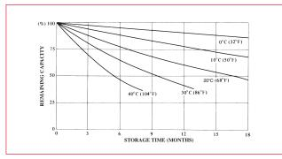
Figure 5. Self Discharge Characteristics
