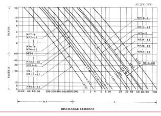
Figure 1. 20-Hour Rate Capacity Selection Chart
