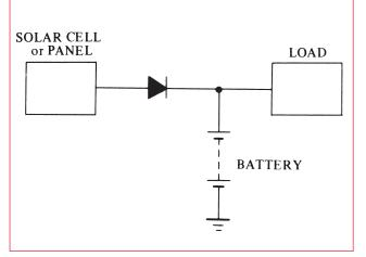
Figure 15. Block Diagram of a Solar System
